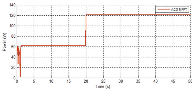
Fig.14. ACO Power curve under rapid variation of irradiance
