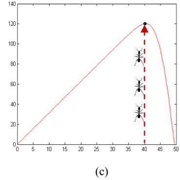
Fig.7. (c) Ants move towards the optimized point, i.e. the MPP
