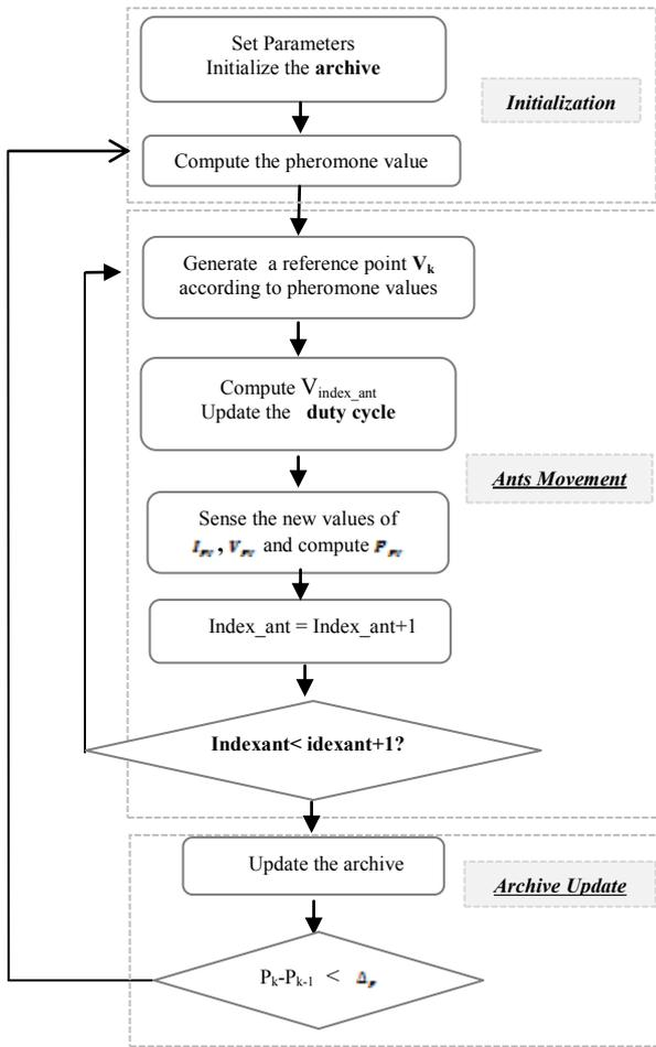
Fig.6. Flow chart of ACO\_MPPT controller
