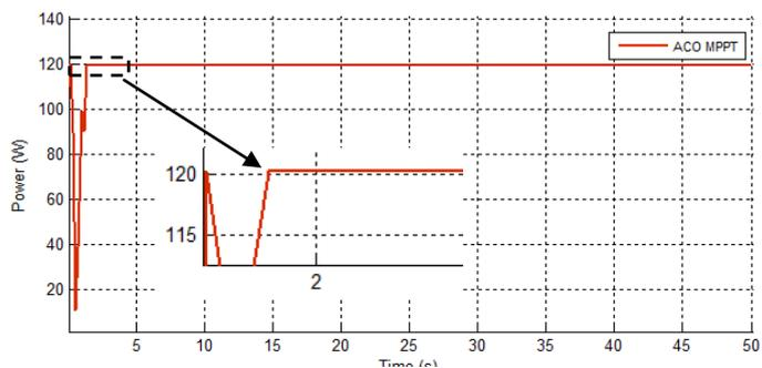
Fig.10. ACO Power curve under STDC (25°C,1000W/m<sup>2</sup>)
