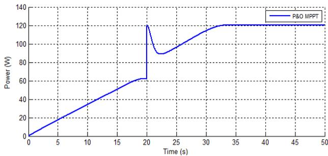
Fig.13. P&O Power curve under rapid variation of irradiance
