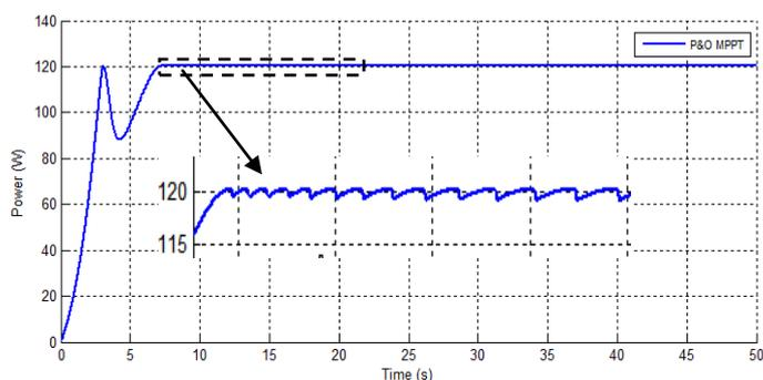
Fig.9. P&O Power curve under STDC (25°C,1000W/m<sup>2</sup>)
