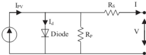
Fig.2 Equivalent circuit of a PV cell
