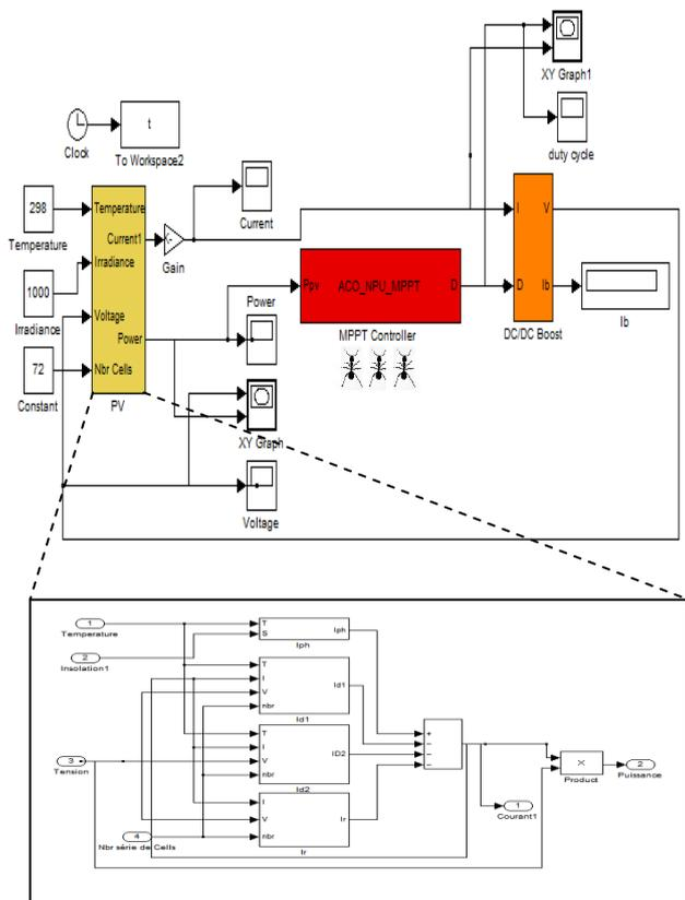
Fig.8. Simulink model of the PV System
