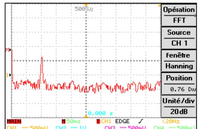
Fig. 7. FFT of ADC1 signal without fault.
