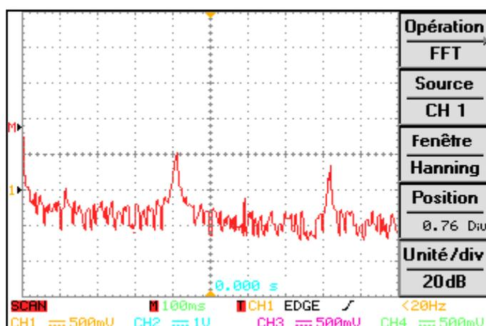
Fig. 9. FFT of ADC1 signal with fault.
