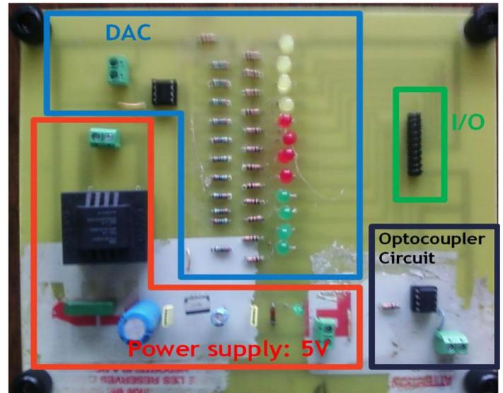
Fig. 5. Picture of the DAC converter.
